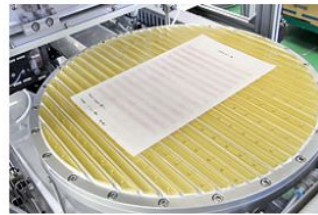
Measure the pressure distribution of cleaning polish against liquid crystal panels
